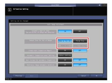
4 Select [OFF] in [Automatic Reprint when Deviation/Out of Range was Detected].
