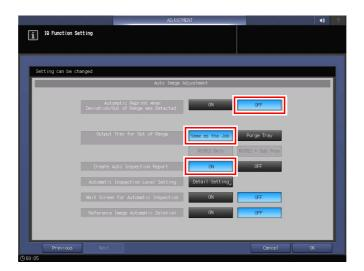
[Automatic Reprint when Deviation/Out of Range was Detected]: [OFF] [Output Tray for Out of Range]: [Same as the Job] [Create Auto Inspection Report]: [ON]
