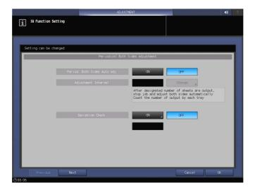
2 Select [Continue Output] in [Operation after Deviation/Out of Range was Detected], and type "00" for [Detection Count] using the keypad on the screen.
