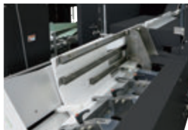
Rotary Grip Style Cover Feeder with Lower Table (SB-17)
