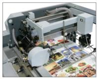
mechanism feeds individual sheets into the SmartStacker for finishing.
