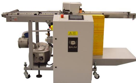
The Baum 20 IPF Independent Pile feeder is a heavy duty, mobile independent pile feeder which allows you to load up to 25" of material on the feeder. It has a precision register table and a state of the art control system.
