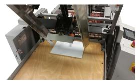
Two sided funnel design is a standard feature. A height sensor reads the stack height and automatically moves the lift down to keep receiving more sheets until the maximum limit is reached.
