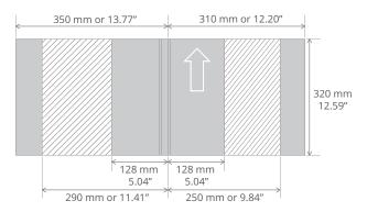
Maximum Cover Sheet Fore-edge Length: 660 mm or 25.98" (Up to 350 mm or 13.77" towards from the clamp face, and up to 310 mm or 12.20" backwards from the clamp face.) Additional two scoring lines for flap cover can be made in ////// range.
